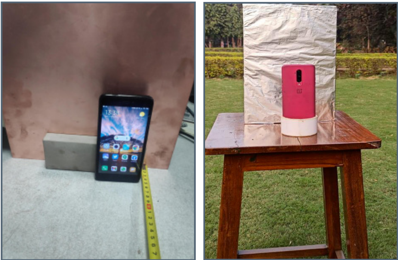
Figure 1.3: Two examples of metallic back reflectors, (a) metal plate and (b) aluminium foil, with transmitter phones on non-metallic supports.
