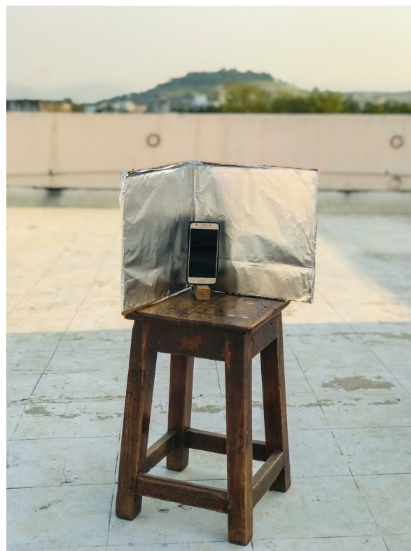
Figure 1.4: Set-up of Corner reflector antenna with the radiator (Smartphone) at the centre
