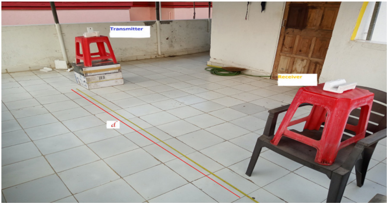
Figure 2.1: An example of transmitter/receiver locations relative to floor and walls
